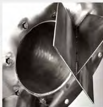
The material deflector directs material flow to minimize material carryover
