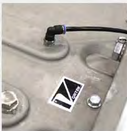
The air purge is used to pressurize the bonnet and keep material in the flow stream
