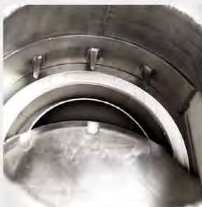
The silicone blade seal is recessed to protect it from material flow and to reduce wear
