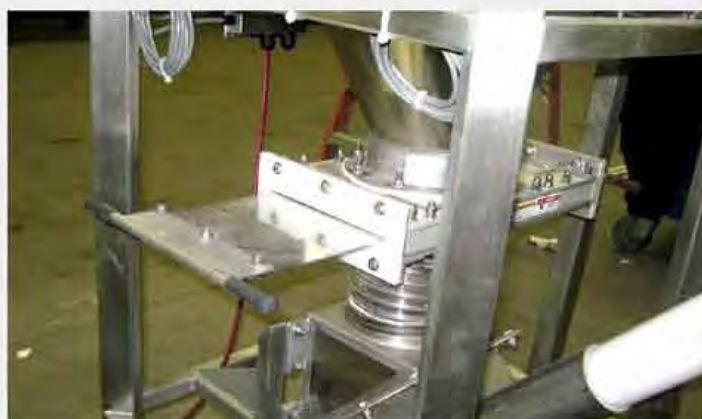
6" (152mm) Hand Slide Orifice Gate as isolation valve above a flexible screw conveyor
