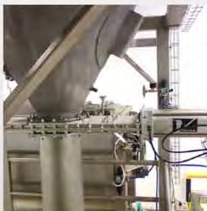
10" (254mm) Quantum Orifice Gate handling cement powder
