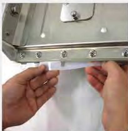
Shim removal for seal adjustment while valve is in-line
