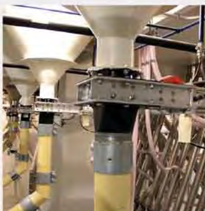
6" (152mm) Roller Gate below hopper handling flour
